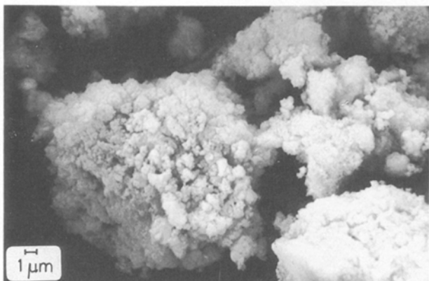
Figure 6 SEM photomicrograph and EDX analysis for the sample treated at 500 °C TiO_2 27.3%, ZrO_2 72.7%.
