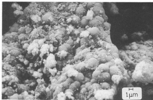
Figure 7 SEM photomicrograph and EDX analysis for the sample treated at 800 °C: TiO_2 50.95%, ZrO_2 49.05%.
